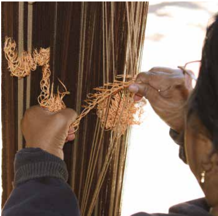
A Guaraní weaver prepares the heddles of her loom to carry out the technique of karakarapepo . Photograph: Elvira Espejo
