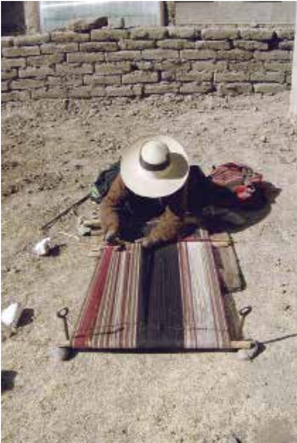
The horizontal or four-stake loom, in the Infotambo-Challapata project. Photograph: Elvira Espejo
